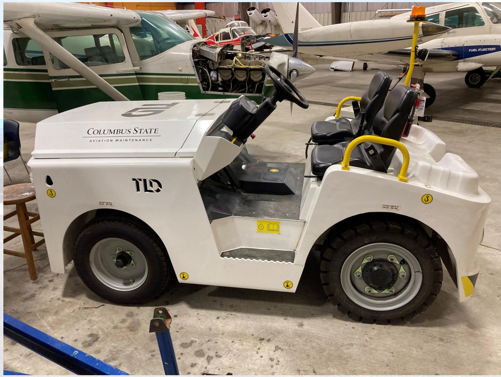
Aircraft Tug - special, low-profile vehicle to move aircraft
